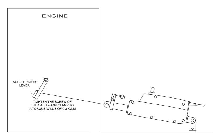
DO NOT MOUNT THE ACTUATOR WHERE ITCOULD BE SUBJECTED TO KNOCKS OR STRONG VIBRATIONS. DO NOT MOUNT IN A WAY THAT COULD CREATE DANGEROUS SITUATIONS.
