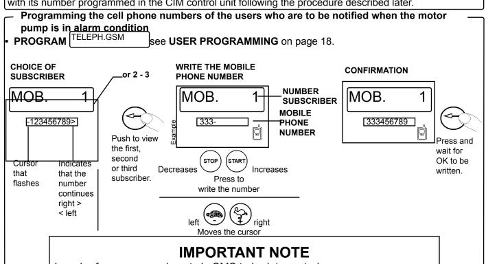
In order for a command sent via SMS to be interpreted correctly, it is important to programme the telephone number exactly as it is given by the mobile telephone network, and therefore inclusive of international dialling code and without the first zero of the dialling code (if there is one) of the telephone company.
